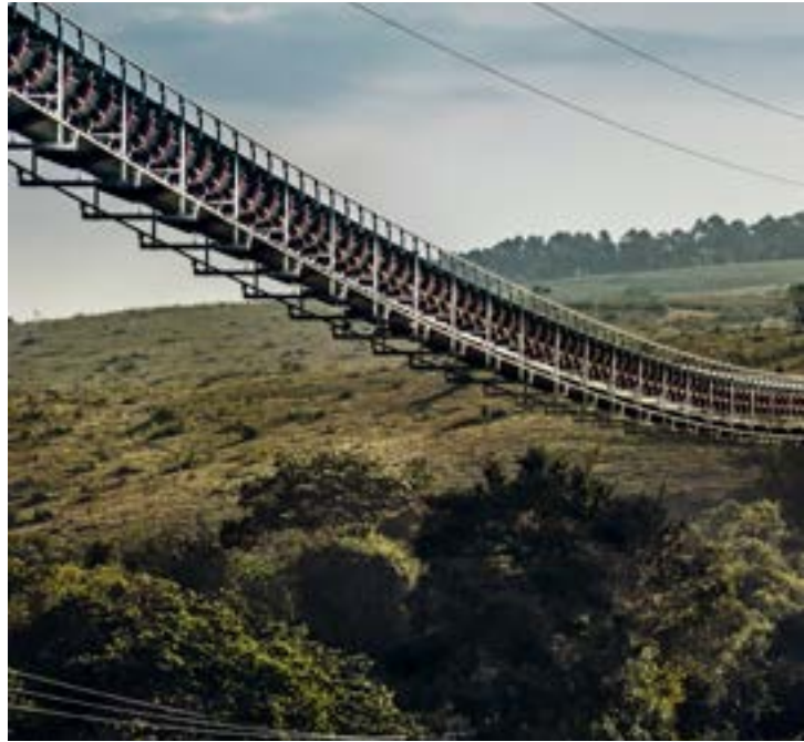
The flying belt transports thousands of tons of limestone per hour in the Brazilian highlands.
